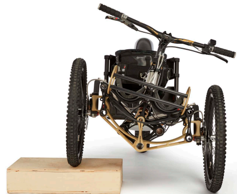
Icon "Carver" articulating front end rises over obstacles, keeping seat and rider upright.
